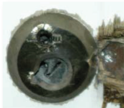
7.62 X 51 (FB7) embedded in cylinder guard
